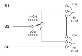
Figure 25. Adjustable Speeds Using Potentiometers In Series
