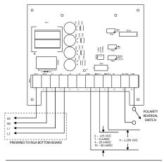
Figure 10. RGA403 Analog Input Signal Connections
