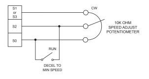
Figure 18. Run/Decelerate to Minimum Speed Switch
