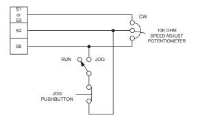
Figure 30. RUN/JOG Switch - Speed Adjust Potentiometer Connection
