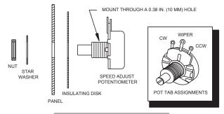
Figure 6. Speed Adjust Potentiometer
