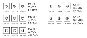
Figure 20. Recommended FWD TQ, REV TQ, and IR COMP settings (actual settings may vary with each application)
