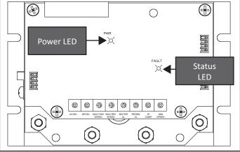
Minimum Speed (MIN SPD): The MIN SPD setting determines the minimum motor speed when the speed adjust potentiometer is set for minimum speed. It is factory set for zero speed. To calibrate the MIN SPD:
