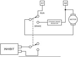
Figure 7. Dynamic Brake Wiring
