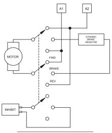
Figure 17. Reversing Circuit Wiring
