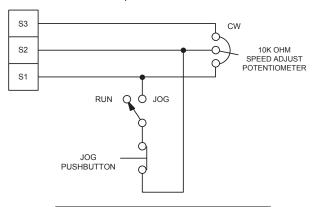
Figure 14. RUN/JOG Switch - Potentiometer Connection
