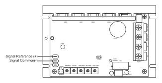
Figure 4. Analog Input Signal Connections
