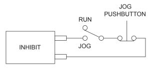
Figure 13. RUN/JOG Switch - Inhibit Connection
