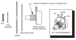
Figure 3. Speed Adjust Potentiometer
