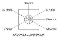
Figure 9. Recommended CURRENT LIMIT Settings
