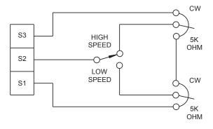
Figure 11. Adjustable Speeds Using Potentiometers In Series
