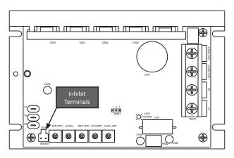
Figure 8. Inhibit Terminals
