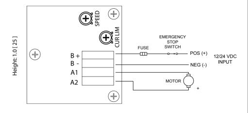
**STEP 1: Wiring**. Connect motor terminals to A1 and A2 (with A1 being positive). Connect DC input power to B+ and B-.
