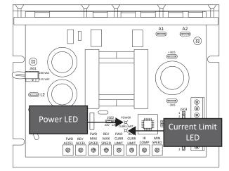
Minimum Speed (MIN SPD): The MIN SPD setting determines the motor speed when the drive is commanded a minimum speed (potentiometer full CCW or 0 VDC). It is factory set for zero speed. To calibrate the MIN SPD:
