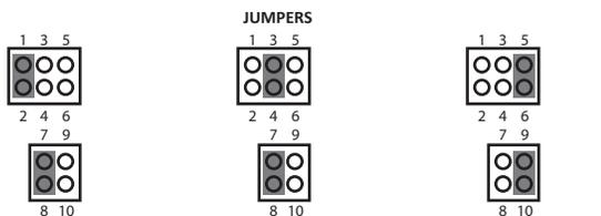
0 to ± 5 VDC or Potentiometer Jumper Pins 1&2 and 7&8      0 to ± 10 VDC Jumper Pins 3&5 and 7&8      4-20 mA Jumper Pins 5&6 and 9&10
