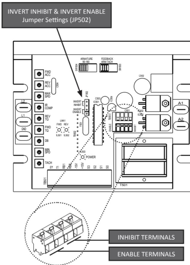
Figure 15. Inhibit / Enable Locations
