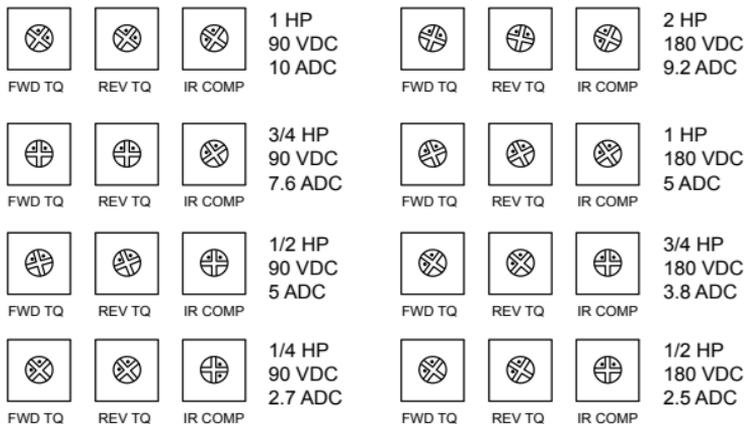
Figure 16. Recommended FWD TQ, REV TQ, and IR COMP Settings
