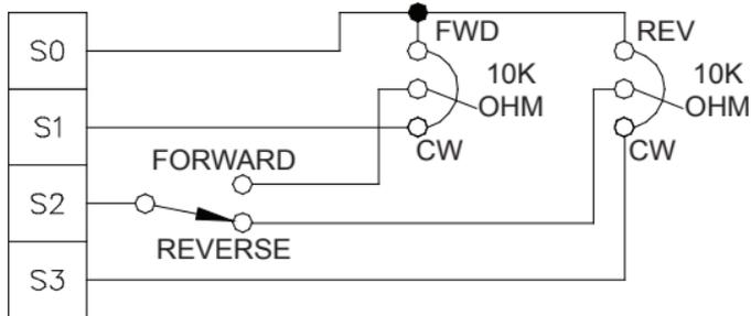
Figure 24. Independent Adjustable Forward and Reverse Speeds
