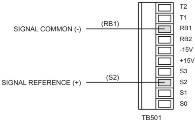
Figure 9. Analog Input Signal Connections
