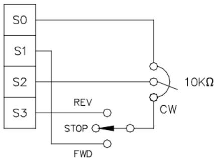
Figure 19. Forward-Stop-Reverse Switch
