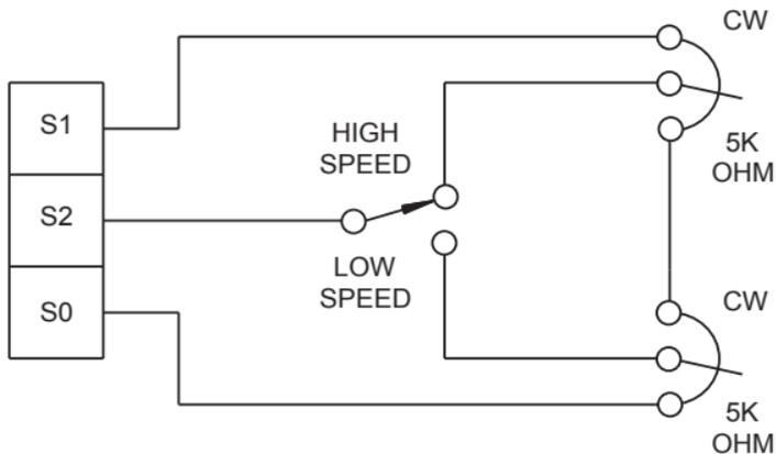
Figure 22. Adjustable Speeds Using Potentiometers In Series
