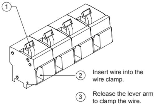
Figure 6. Cage Clamp Terminal Block
