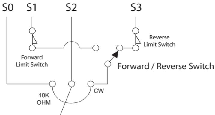
Figure 20. Direction Switch With End Of Travel Limit Switches
