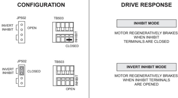
Figure 11. Inhibit Switch Settings
