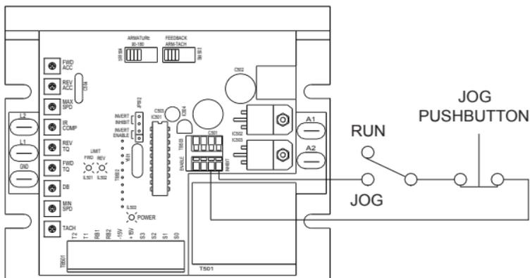
Figure 26. RUN/JOG Switch - Inhibit Connection
