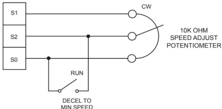
Figure 13. Run/Stop Switch
