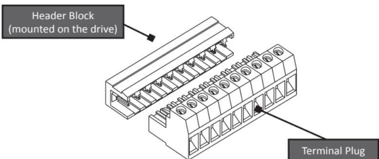
Figure 5. Quick Disconnect Terminal Block
