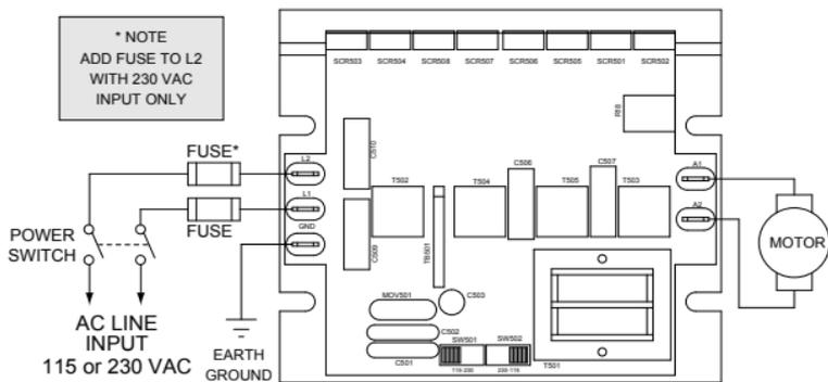
Figure 7. Power and Motor Connections (bottom board)
