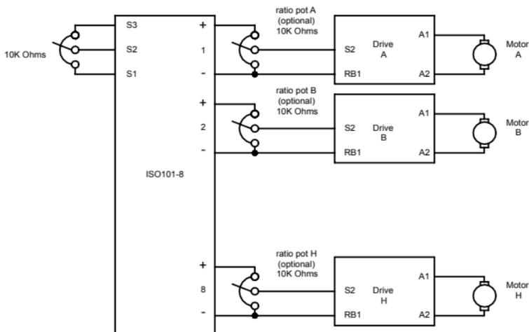
Figure 29. Single Speed Potentiometer Control of Multiple Drives
