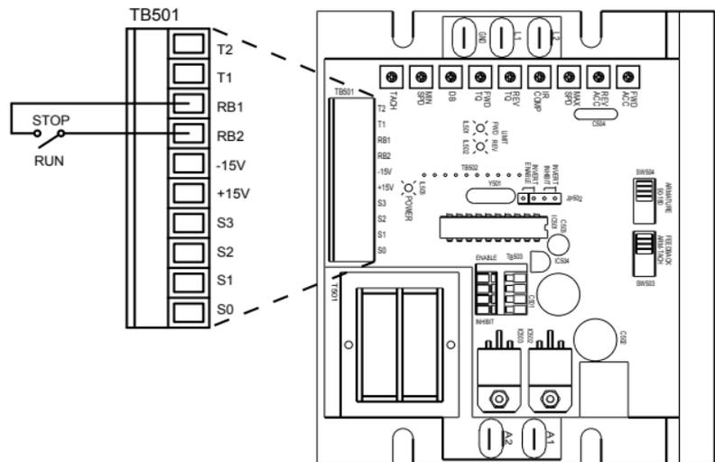
Figure 12. Regenerative Brake Switch
