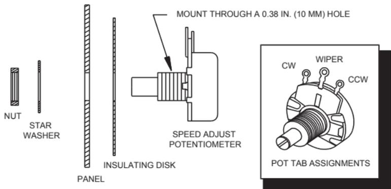
Figure 4. Speed Adjust Potentiometer
