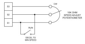
Figure 16. Run/Decelerate to Minimum Speed Switch
