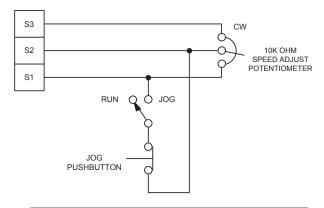
Figure 25. RUN/JOG Switch - Connection to Speed Adjust Potentiometer
