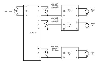
Figure 27. Single Speed Potentiometer Control of Multiple Drives
