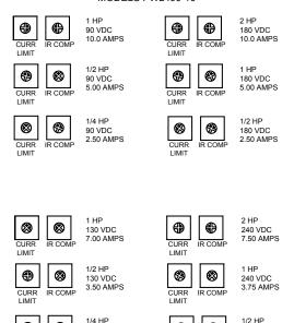
Figure 19. Recommended CURR LIMIT and IR COMP Settings for model PWL400-10
