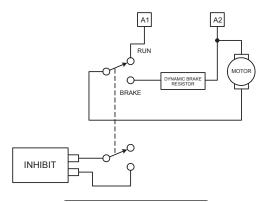
Figure 14. Dynamic Brake Wiring
