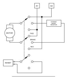
Figure 28. Reversing Circuit Wiring
