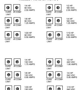
Figure 17. Recommended CURR LIMIT and IR COMP Settings for models PWL400-3 and PWL440-3 (actual settings may vary with each application)
