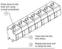
Figure 8. Cage Clamp Terminal Block
