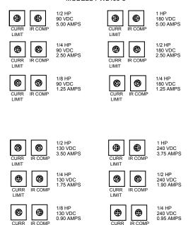
Figure 18. Recommended CURR LIMIT and IR COMP Settings for model PWL400-5
