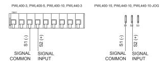
Figure 9. Analog Input Signal Connections
