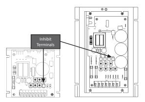
Figure 15. Inhibit Terminals
