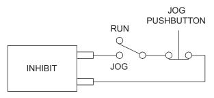
Figure 24. RUN/JOG Switch - Connection to Inhibit Plug
