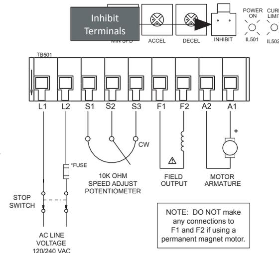
\* NOTE: Do not add fuse to L2 unless input voltage is 230 VAC.
