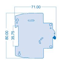
TECHNA'S Rtec range provides combined residual current (earth leak) protection and overload/short circuit protection in a single device and can be used to replace an RCCB/MCB combination.
