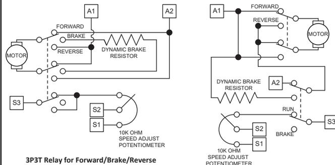
3P3T Relay for Forward/Brake/Reverse
