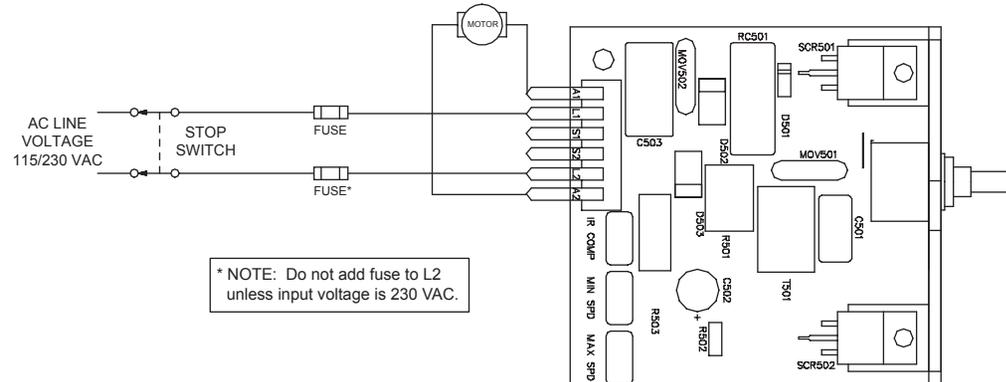
\* NOTE: Do not add fuse to L2 unless input voltage is 230 VAC.
