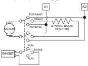
3P3T Relay for Forward/Brake/Reverse
