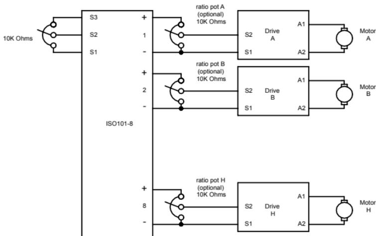
Figure 18. Single Speed Potentiometer Control of Multiple Drives
