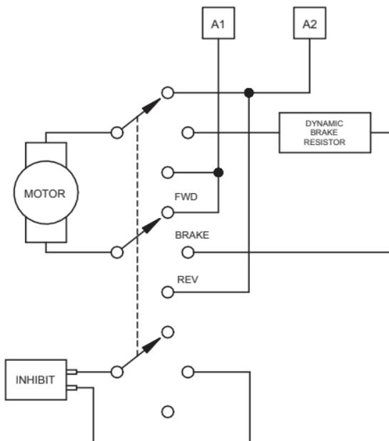
Figure 19. Reversing Circuit Wiring
