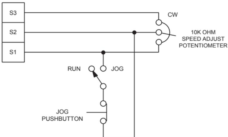
Figure 16. RUN/JOG Switch - Connection to Speed Adjust Potentiometer
