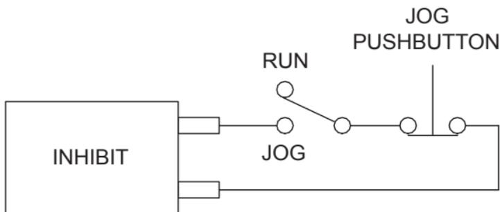
Figure 15. RUN/JOG Switch - Connection to Inhibit Plug
