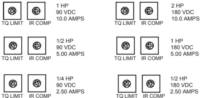
Figure 11. Recommended TQ LIMIT and IR COMP Settings
