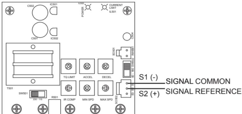
Figure 5. Analog Input Signal Connections (PAT440 and PAT450)
