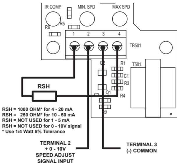
Figure 6. Analog Input Signal Connections (PAT443)
