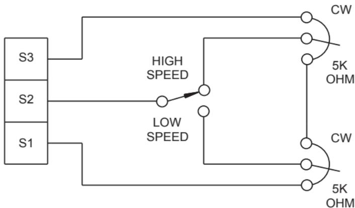
Figure 13. Adjustable Speeds Using Potentiometers In Series
