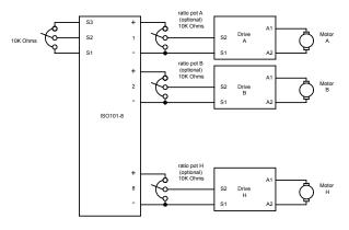
Figure 18. Single Speed Potentiometer Control of Multiple Drives
