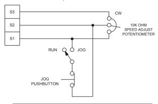
Figure 16. RUN/JOG Switch - Connection to Speed Adjust Potentiometer
