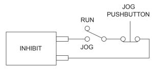
Figure 15. RUN/JOG Switch - Connection to Inhibit Plug
