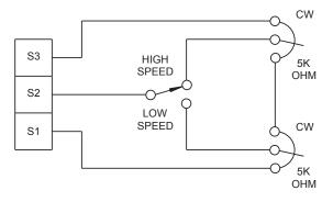
Figure 13. Adjustable Speeds Using Potentiometers In Series
