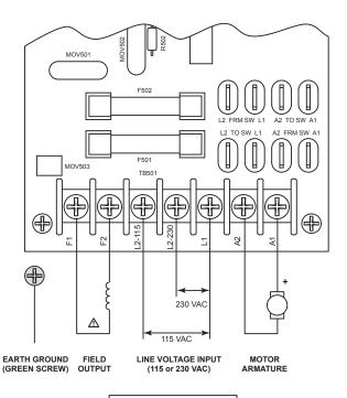
NOTE: DO NOT make any connections to F1 and F2 if using a permanent magnet motor.
