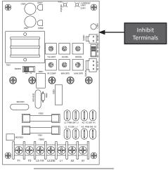
Figure 9. Inhibit Terminals
