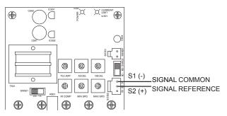
Figure 5. Analog Input Signal Connections (PAT440 and PAT450)
