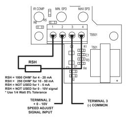
Figure 6. Analog Input Signal Connections (PAT443)
