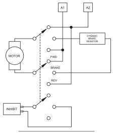
Figure 19. Reversing Circuit Wiring
