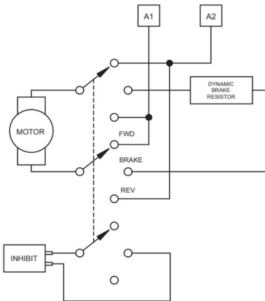
Figure 19. Reversing Circuit Wiring
