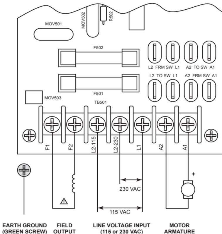
**NOTE: DO NOT** make any connections to F1 and F2 if using a permanent magnet motor.
