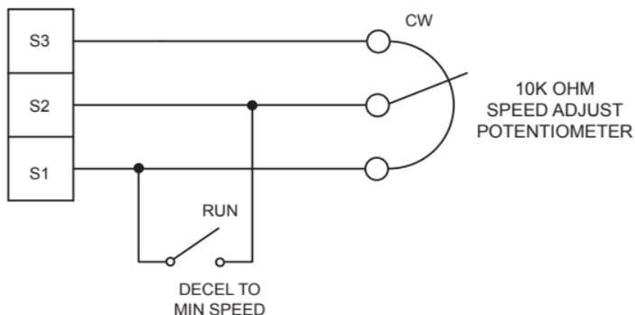
Figure 10. Run/Decelerate to Minimum Speed Switch
