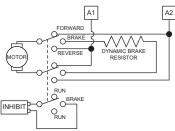
3P3T Relay for Forward/Brake/Reverse
