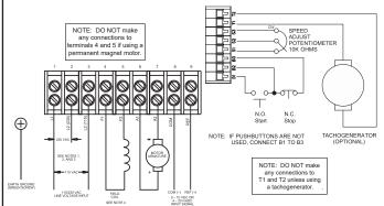
MHS443 series drives are pre-installed with a 10K ohm, 1/4 W potentiometer for speed control.
