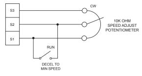
Figure 12. Run/Decelerate to Minimum Speed Switch
