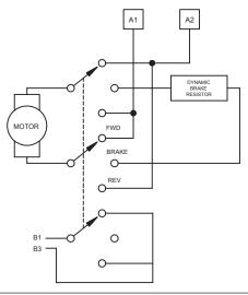
Figure 21. Reversing Circuit Wiring with no 3-Wire Start/Stop
