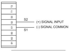
Figure 6. Analog Input Signal Connections
