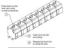
Figure 5. Cage Clamp Terminal Block
