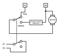
Figure 11. Dynamic Brake Wiring with no 3-Wire Start/Stop
