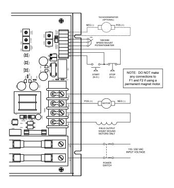
Figure 8. MM501U Connections
