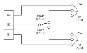
Figure 16. Adjustable Speeds Using Potentiometers In Series
