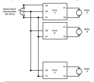
Figure 20. Single Speed Potentiometer Control of Multiple Drives
