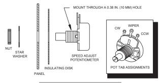
Figure 4. Speed Adjust Potentiometer
