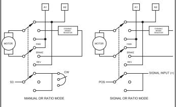
Signal Minimum (SIG MINI): The SIG MINI setting determines the minimum motor speed when the input voltage or current signal is set for minimum speed. It only comes into effect in Signal or Ratio mode. It is factory set for zero speed. To calibrate the SIG MINI:
