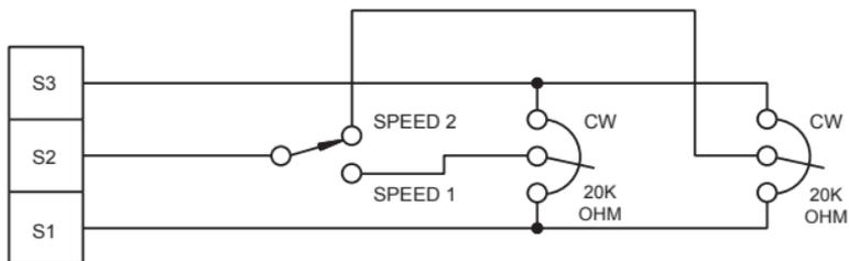
Figure 11. Independent Adjustable Speeds
