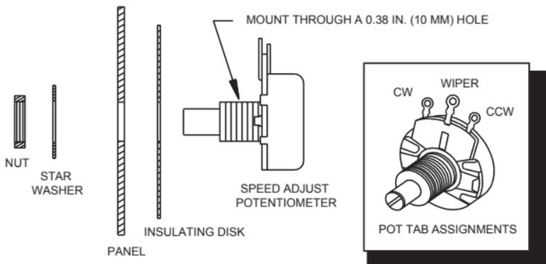
Figure 3. Speed Adjust Potentiometer
