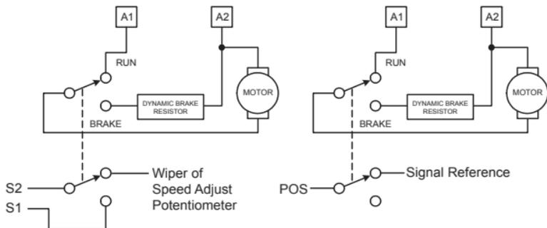
Figure 6. Dynamic Brake Wiring
