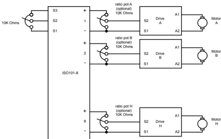
Figure 14. Single Speed Potentiometer Control of Multiple Drives
