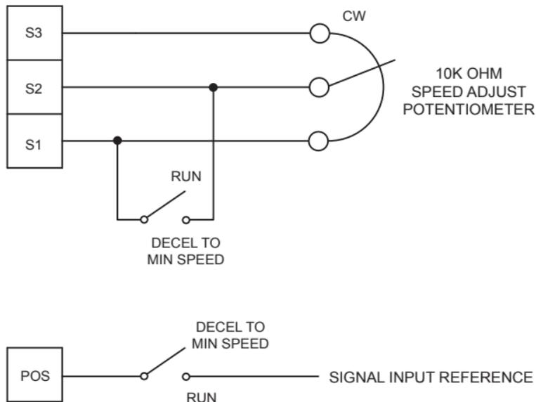
Figure 7. Run/Decelerate to Minimum Speed Switch
