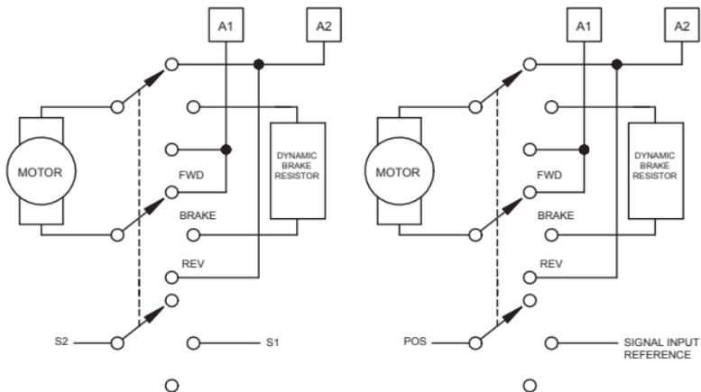
Figure 15. Reversing Circuit Wiring
