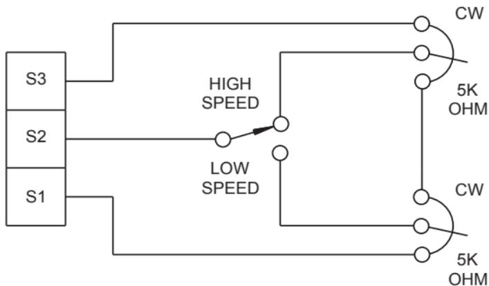
Figure 10. Adjustable Speeds Using Potentiometers In Series
