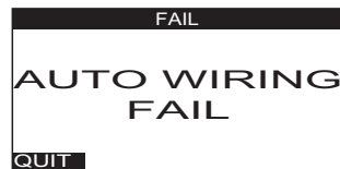
Wiring change failure Press Enter to QUIT
