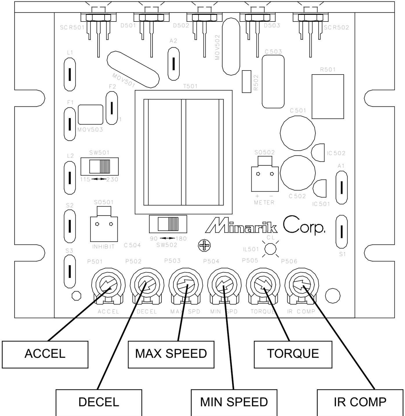
**Figure 10. Calibration Trimpot Layout**
