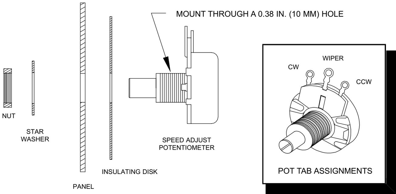
**Figure 3. Speed Adjust Potentiometer**
