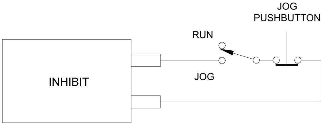
**Figure 15. RUN/JOG Switch Connection to Inhibit Plug**
