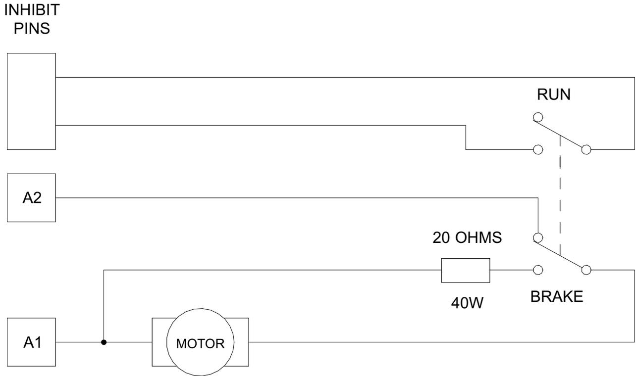
**Figure 9. Dynamic Brake Connections**
