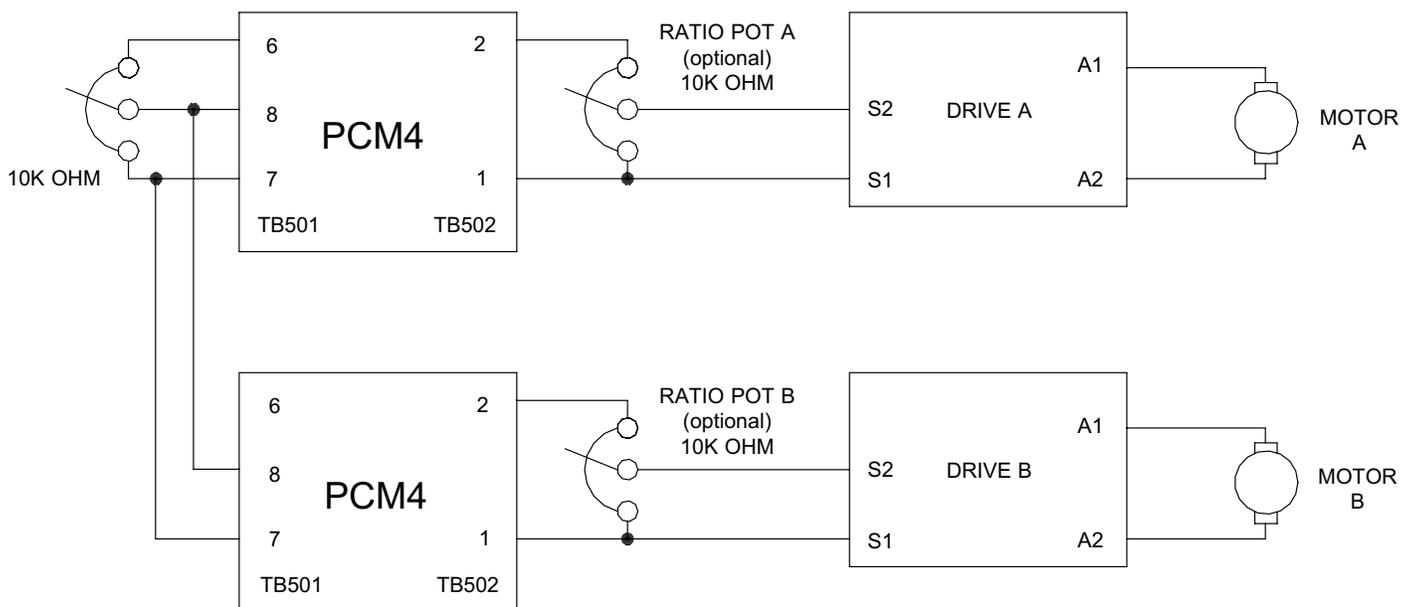
**Figure 18. Single Speed Potentiometer Control of Multiple Drives**
