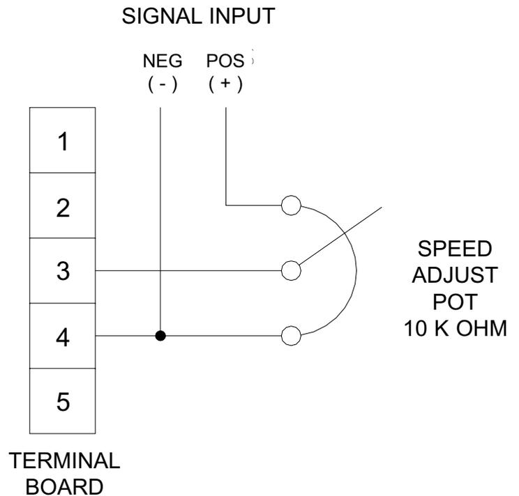
**Figure 5. Voltage Follower Connections With Signal Greater than 3.5VDC**
