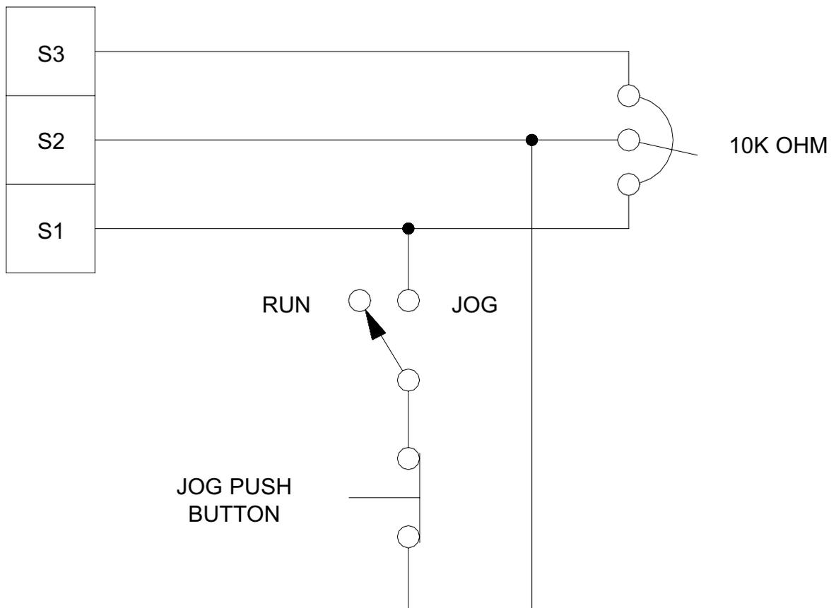
**Figure 16. RUN/JOG Switch Connection to Speed Adjust Potentiometer**
