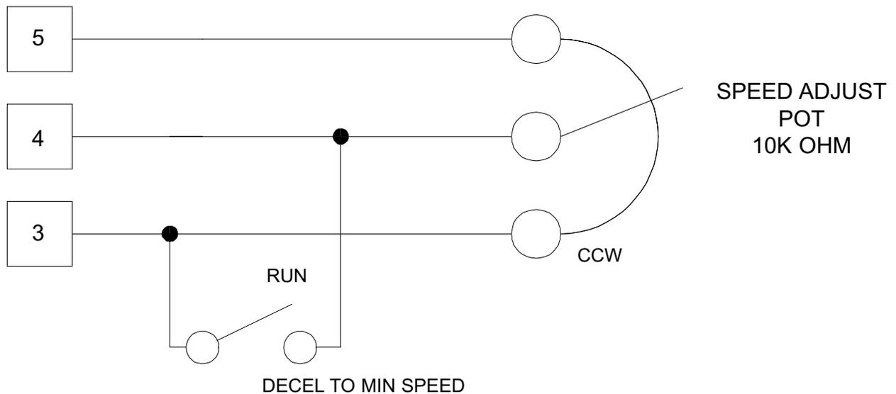
**Figure 8. Run/Decelerate to Minimum Speed Switch**
