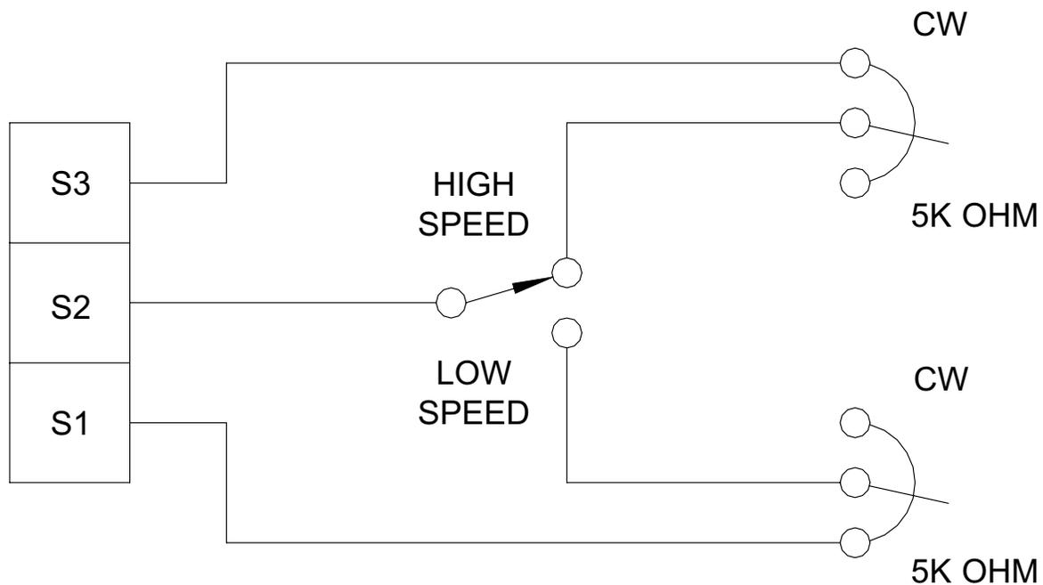
**Figure 13. Adjustable Fixed Speeds Using Potentiometers in Series**
