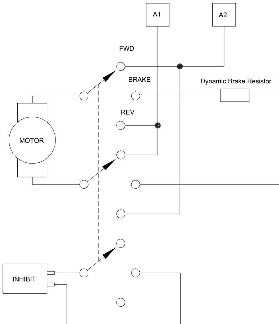
**Figure 19. Reversing Circuit Connection**
