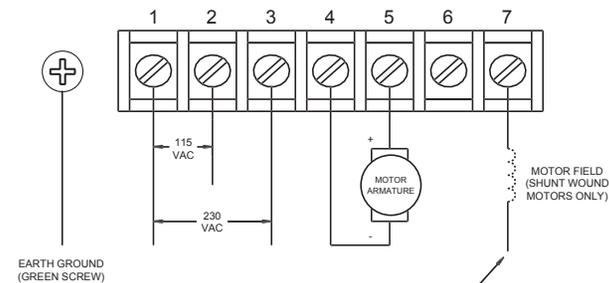
NOTE: DO NOT make any connections to terminals 6 and 7 if using a permanent magnet motor.
