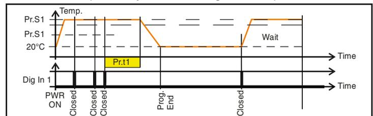
When a new panel is detected before the end of the first soak time, the program restarts and the set point remains equal to Pr.S1.
