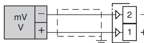
**Input impedance:** > 1 MΩ for mV Input
