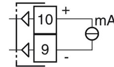
**mA output:** 0/4... 20 mA, galvanically isolated, maximum load resistance: 500Ω.
