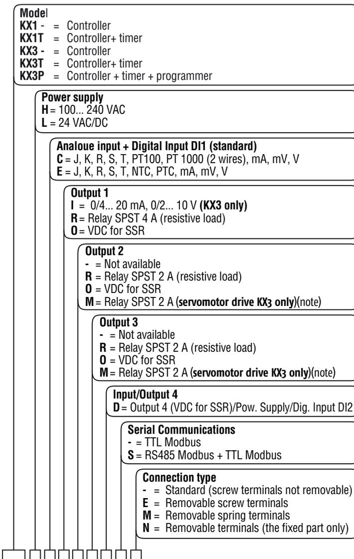
**Note:** For servomotor drive, both **Output 2** and **Output 3** codes must be selected as “**M**”.
