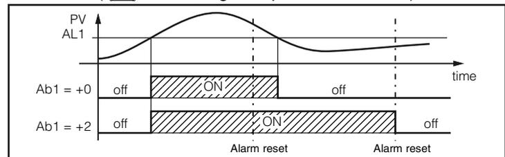
3. An “Acknowledgeable” alarm is an alarm that can be reset even if the conditions that generated the alarm are still present. Alarm acknowledge can be done only by an external command ( button, digital inputs or serial link).
