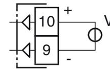
**mA output:** 0/2... 10 V, galvanically isolated, minimum load resistance: 500Ω.
