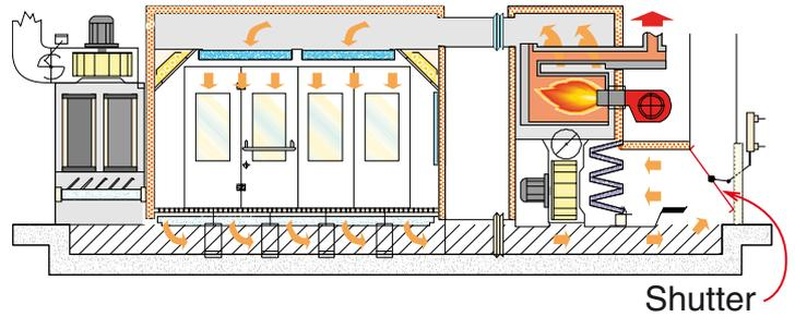
When the drying time is finished, before the operator is allowed to enter into the booth, you must be sure that:
