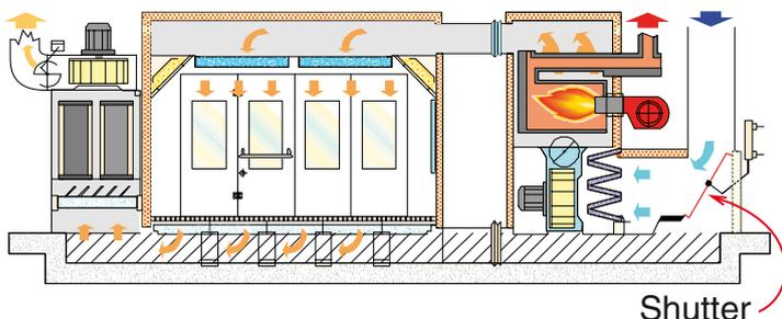
During the passivation and drying phases, the operator is out of the booth and the system closes the shutter of the air and recycles the internal air in order to reduce the power consumption.
