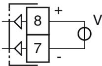
**V output:** 0/2... 10 V, galvanically isolated,  $R_L$  min.: 500Ω.
