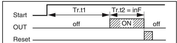
**Delayed start at power up** with a delay time and a "end of cycle" time.
