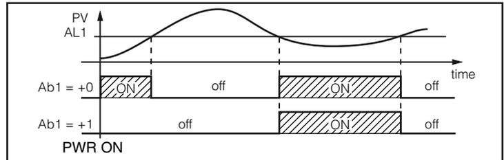
2. A “Latched alarm” (manual reset) is an alarm that will remain active even if the conditions that generated the alarm no longer persist. Alarm reset can be done only by an external command (☐ button, digital inputs or serial link).
