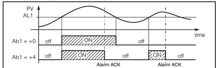
A “relative alarm not active at set point change” is an alarm that masks the alarm condition after a set point change until process variable reaches the alarm threshold  $\pm$  hysteresis.
