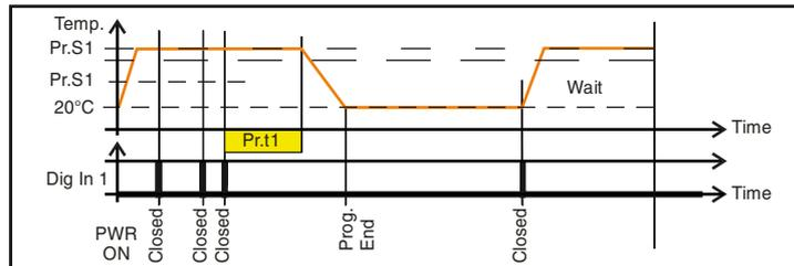
When a new panel is detected before the end of the first soak time, the program restarts and the set point remains equal to Pr.S1.
