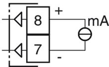
**mA output:** 0/4... 20 mA, galvanically isolated,  $R_L$  max. 600Ω.
