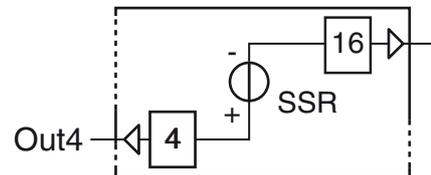
**Logic level 0:**  $V_{out} < 0.5 \text{ VDC}$ ;
