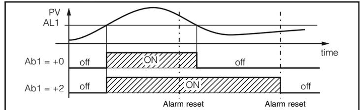
3. An “Acknowledgeable” alarm is an alarm that can be reset even if the conditions that generated the alarm are still present. Alarm acknowledge can be done only by an external command (☐ button, digital inputs or serial link).
