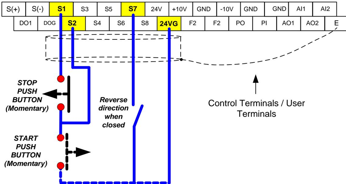
**Note:** Stop mode selection can be set with parameter 07-09, default is **deceleration to stop**.
