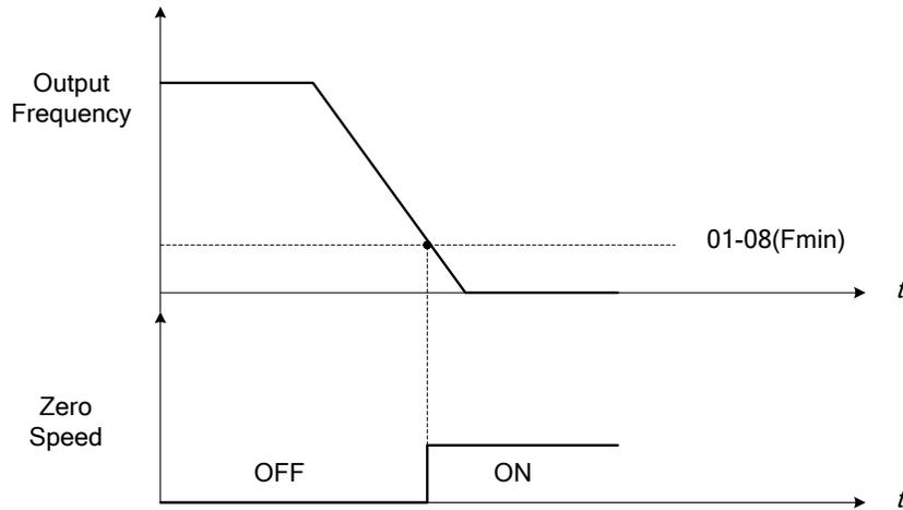
**Figure 4.4.26 Zero-speed operation**
