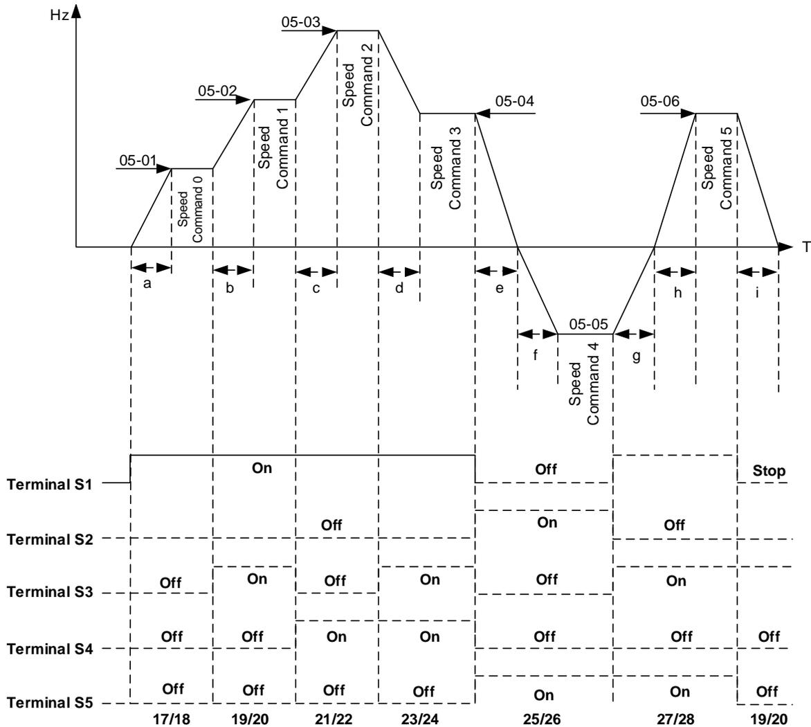
$$a = \frac{(05-17) \times (05-01)}{(01-02)} \quad b = \frac{(05-19) \times [(05-02) - (05-01)]}{(01-02)} \quad c = \frac{(05-21) \times [(05-03) - (05-02)]}{(01-02)} \quad \text{in sec.}$$
