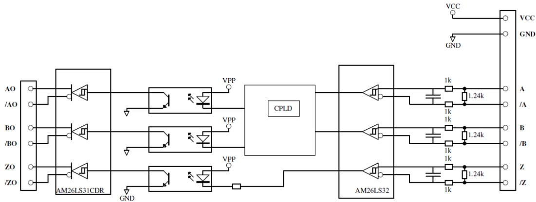
C) JN5-PG-PM speed feedback card: synchronous motor line driver speed feedback card
