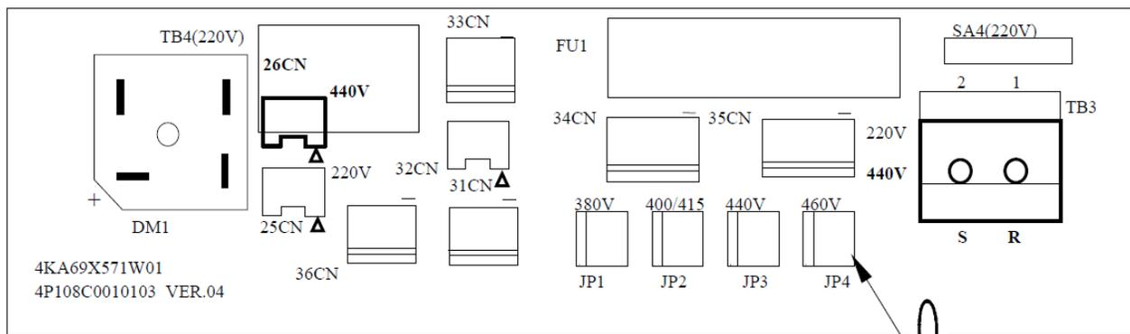
For example, input voltage is 460 Vac, jumper pin needs to put in "460V" position.
