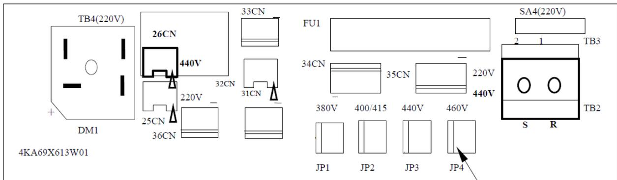
For example, input voltage is 460 Vac, jumper pin needs to put in "460V" position.
