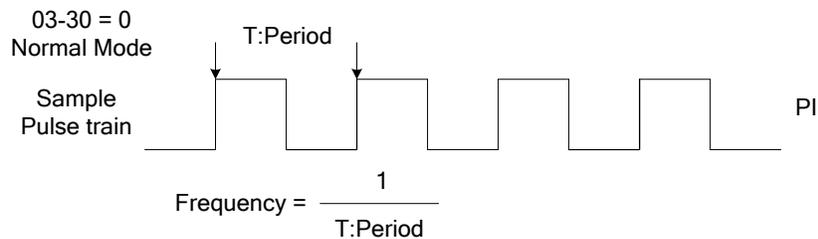
$$\text{Pulse Input Command} = \frac{\text{Frequency}}{\text{Scaling factor (using 03-31)}} \times 100\%(01-02)$$
