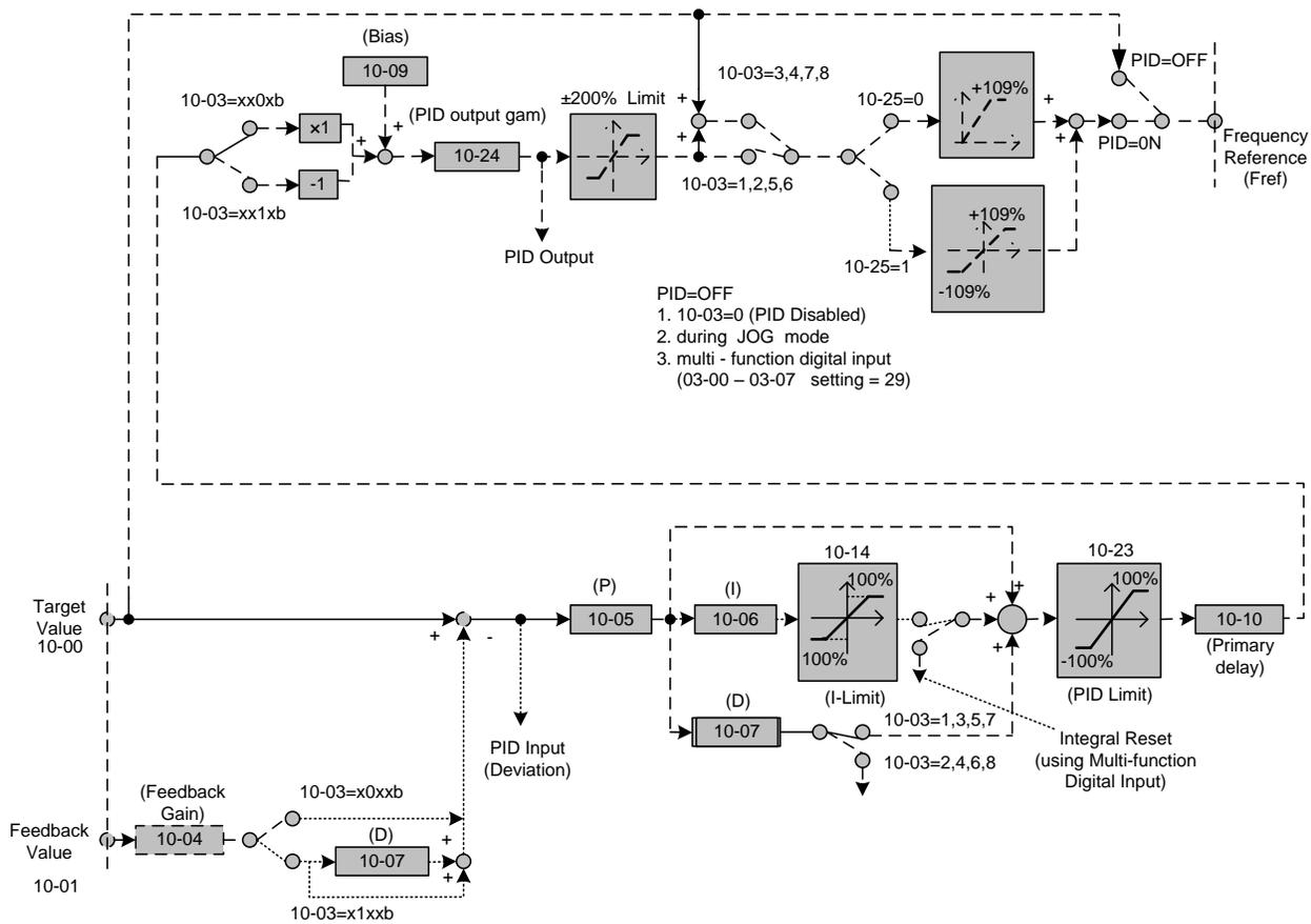
The amplitude of the error can be adjusted with the Proportional Gain parameter 10-05 and is directly related to the output of the PID controller, so the larger gain the larger the output correction.
