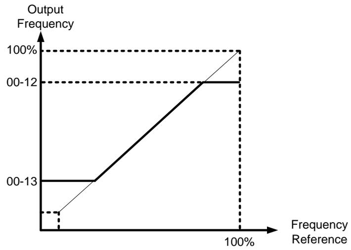
**Figure 4.4.6 Frequency reference upper and lower limits**
