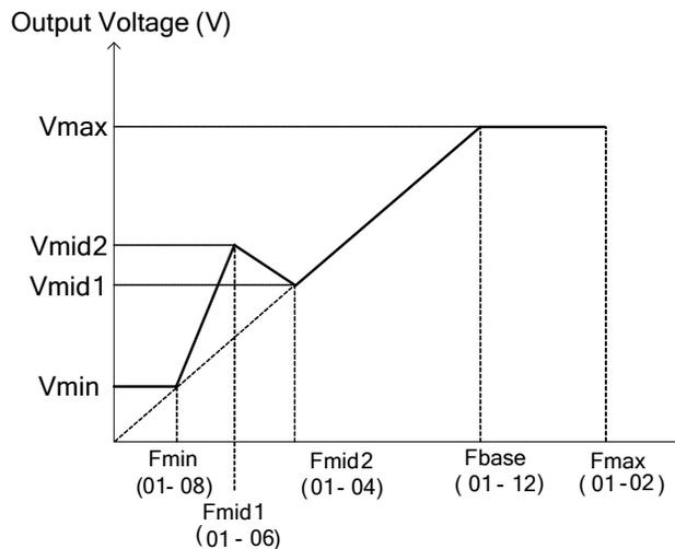
Figure 4.4.13 Torque boosting
