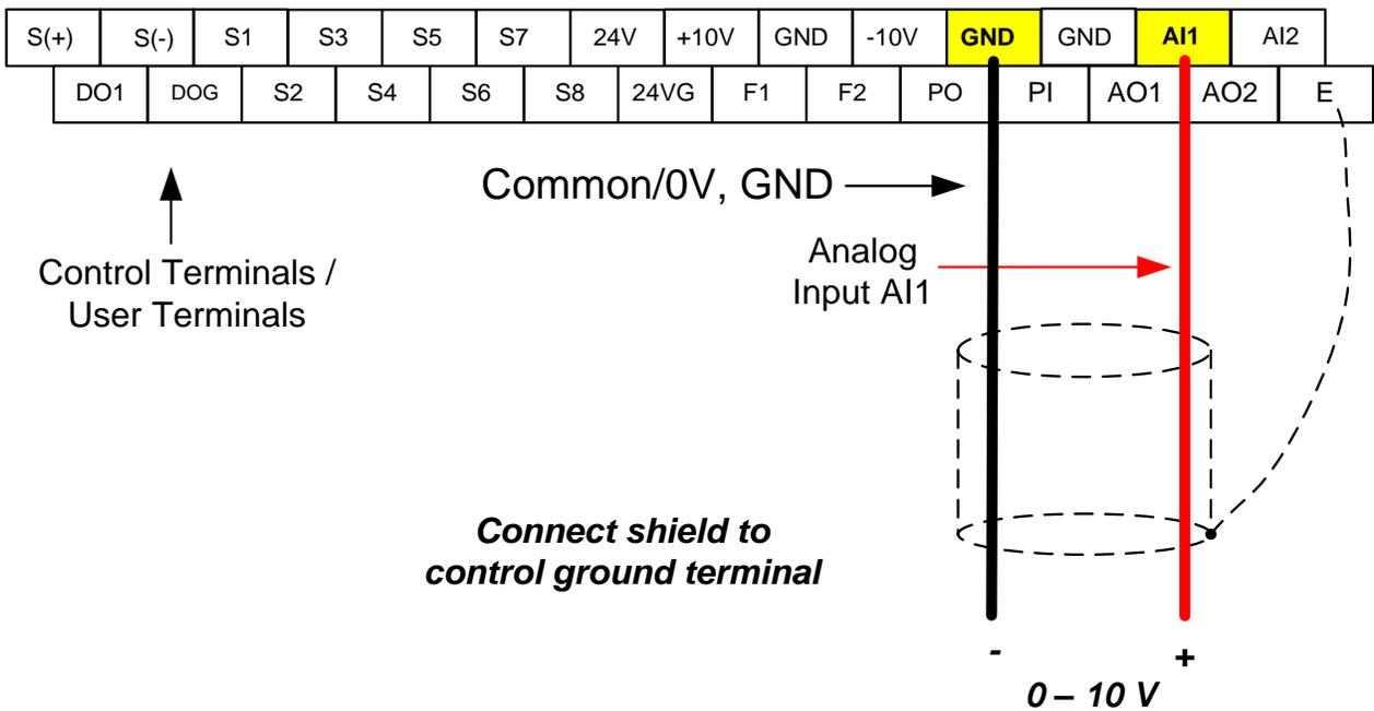
**Analog Reference: Potentiometer / Speed Pot (Setting 00-05 = 1)**
