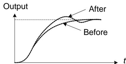
To quickly stabilize the PID control, reduce the integral time (I) and increase the differential time (D) in case overshoot occurs.
