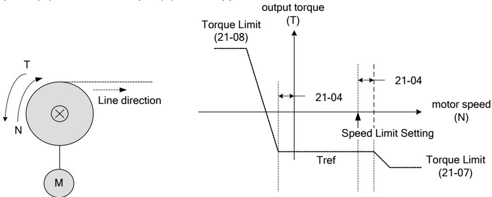
**Figure 4.4.125 Unwind operation**
