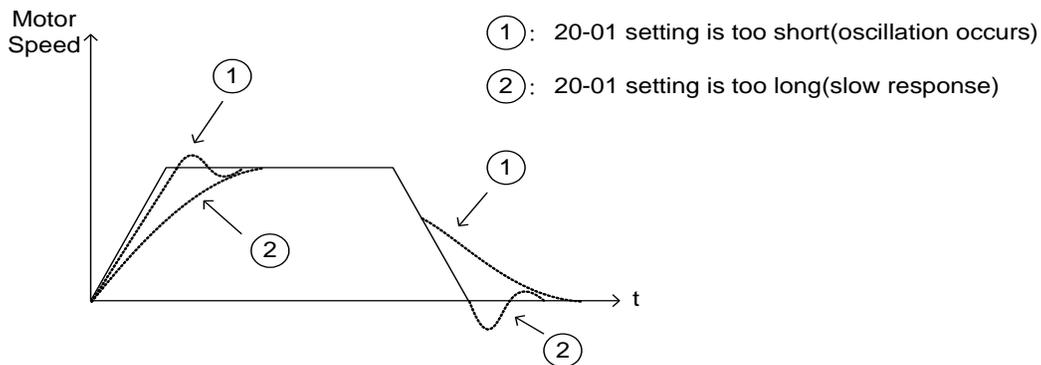
**Figure 4.4.114 The response of ASR integral time**
