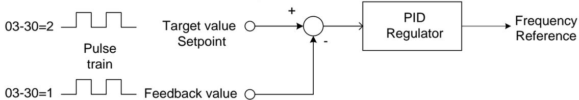
**Figure 4.4.28 PID control**
