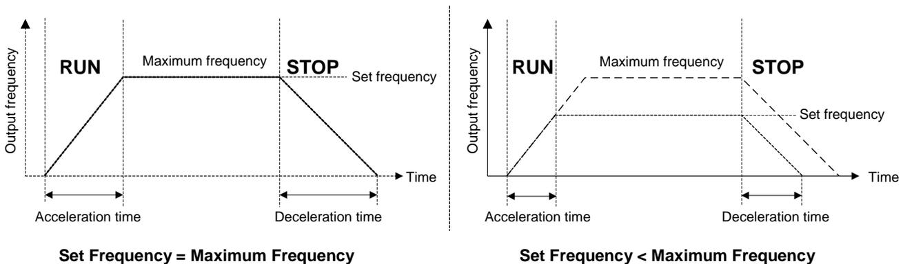
**Note:** If the set acceleration and deceleration times are set too low, the torque limiting function or stall prevention function can become activated if the load torque and or inertia are relatively high. This will prolong the acceleration and or deceleration times and not allow the set times to be followed. In this case the acceleration and or the deceleration times should be adjusted.
