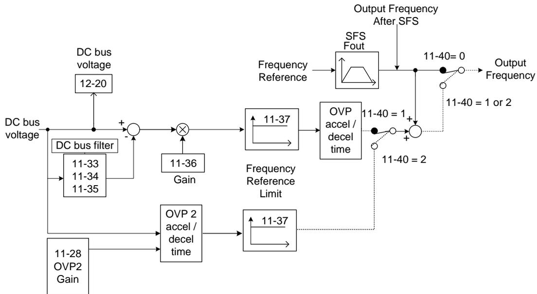
**Figure 4.4.91 OVP operation**
