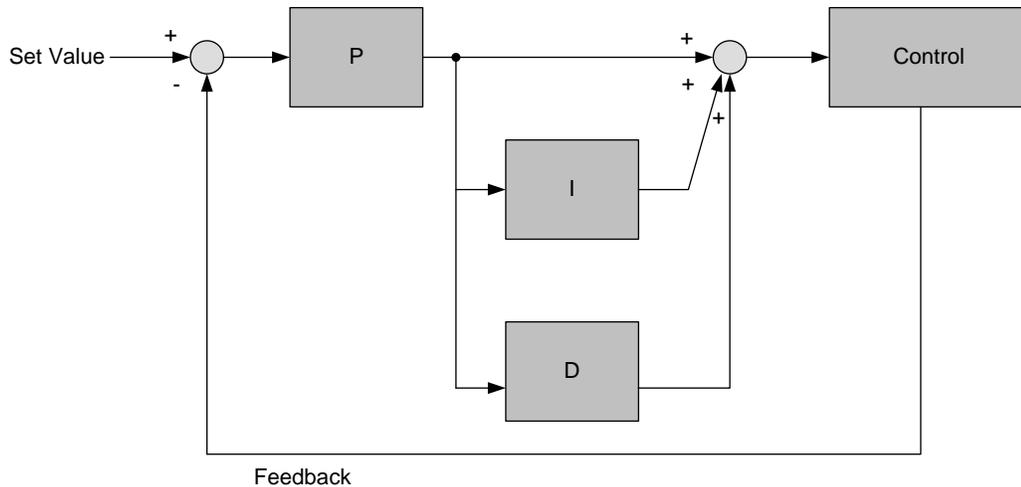
Figure 4.4.79 Basic PID control
