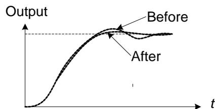
Adjust the integral time (I) in case of long-periodical system oscillation.
