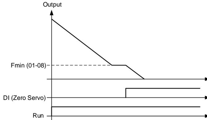
**Figure 4.3.129 Zero-servo positioning**
