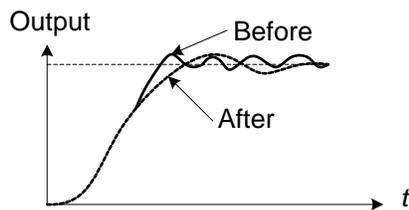
Adjusting the differential time (D) and proportional (P) gain when experiencing short-periodical oscillation.
