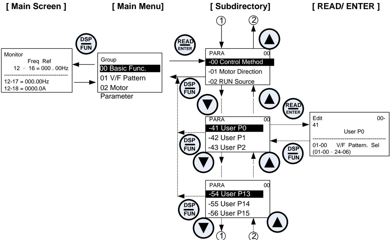
Note: User level (13-06=1) can be set by one or more parameters in the user parameters of 00-41 ~ 00-56.
