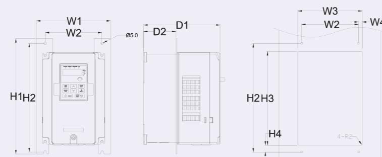
Flange mounting of 3PH 380V 4-75kW and 3PH 220V 1.5-7.5kW VFDs
