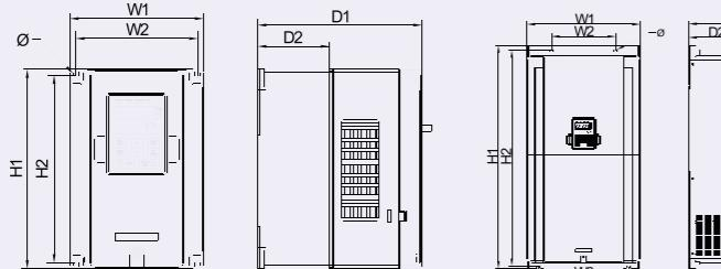
Wall mounting of 3PH 380V 4-37kW and 3PH 220V 1.5-7.5 kW VFDs
