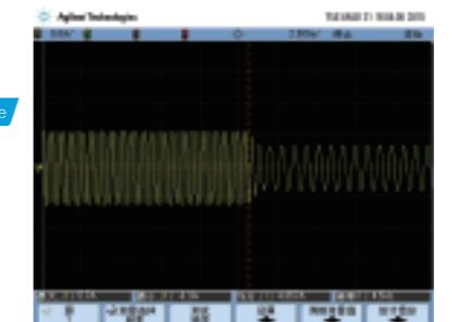
Current waveforms when sudden unloading in vector control mode with 0.5Hz and full load
