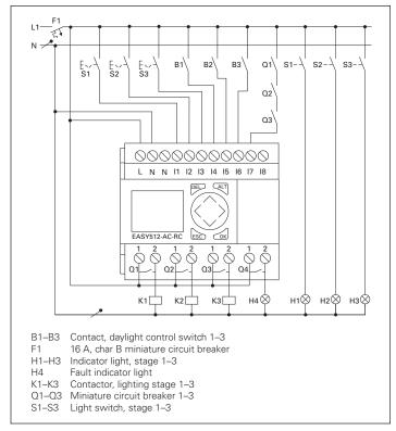
Figure 24. Control Wiring Diagram
