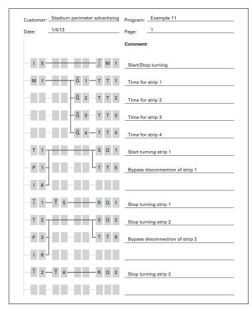
Figure 63. easyRelay Display Diagram
