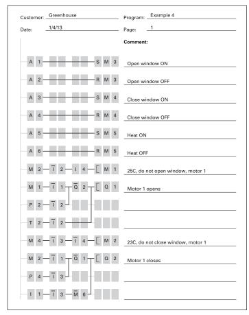
Figure 20. easyRelay Display Diagram
