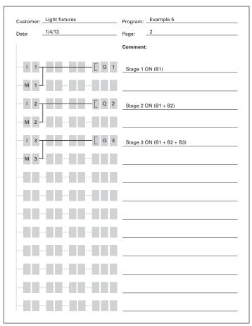
Figure 28. easyRelay Display Diagram
