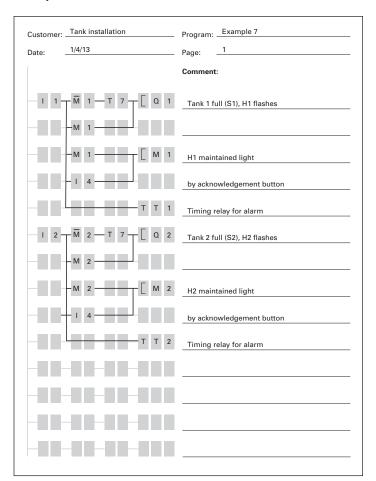
Figure 40. easyRelay Display Diagram
