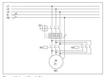
Figure 68. Load Circuit Diagram
