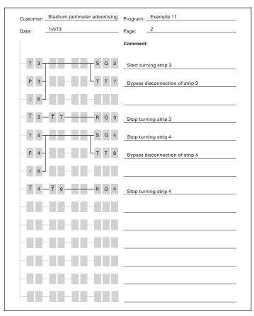
Figure 64. easyRelay Display Diagram
