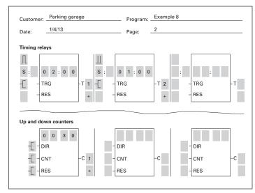
Figure 46. easyRelay Display Parameters
