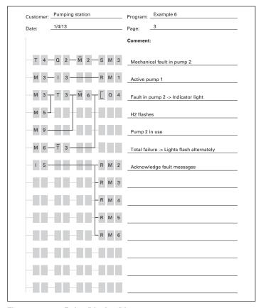
Figure 36. easyRelay Display Diagram
