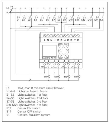
Figure 6. Control Wiring Diagram
