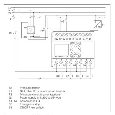
Figure 56. Control Wiring Diagram
