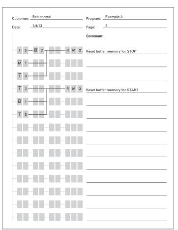
Figure 15. easyRelay Display Diagram
