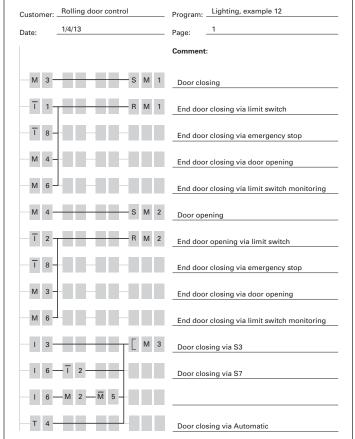
Figure 69. easyRelay Display Diagram
