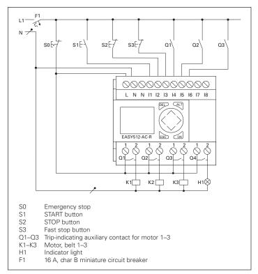
Figure 11. Control Wiring Diagram
