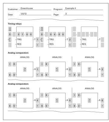
Figure 22. easyRelay Display Parameters
