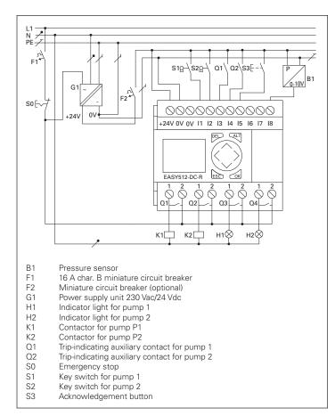
Figure 31. Control Wiring Diagram
