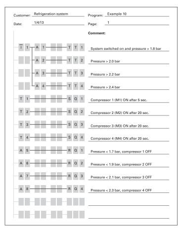
Figure 58. easyRelay Display Diagram
