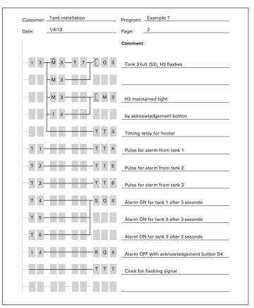
Figure 41. easyRelay Display Diagram
