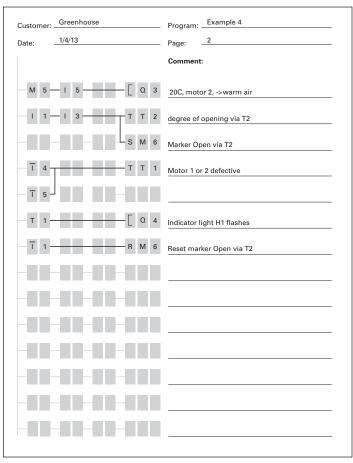
Figure 21. easyRelay Display Diagram
