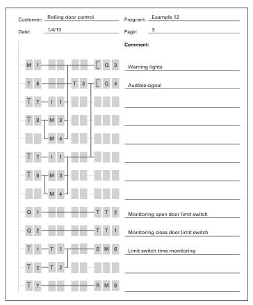
Figure 71. easyRelay Display Diagram
