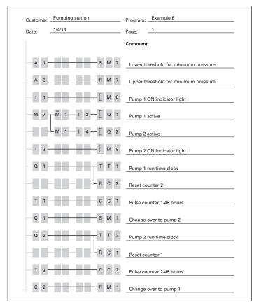
Figure 34. easyRelay Display Diagram
