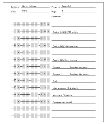
Figure 49. easyRelay Display Diagram
