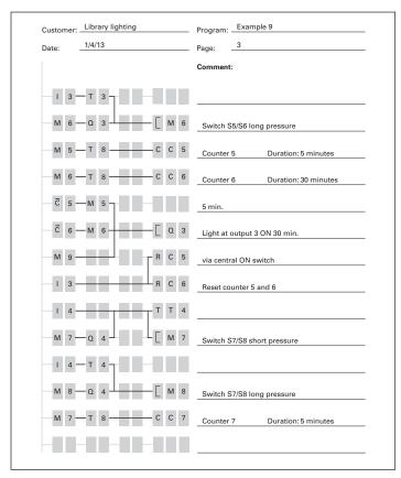
Figure 51. easyRelay Display Diagram
