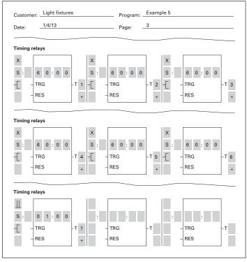
Figure 29. easyRelay Display Parameters
