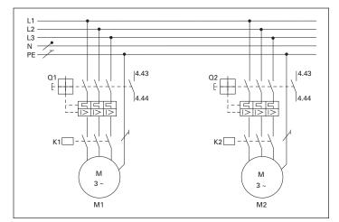
Figure 32. Load Circuit Diagram
