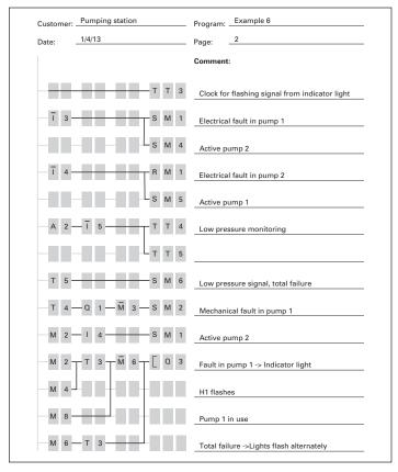
Figure 35. easyRelay Display Diagram
