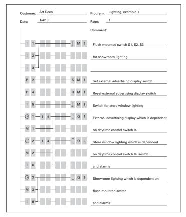
Figure 3. easyRelay Display Diagram
