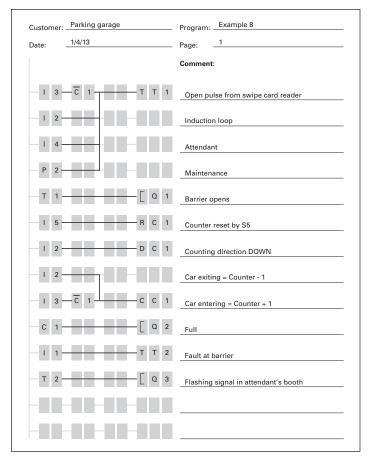
Figure 45. easyRelay Display Diagram
