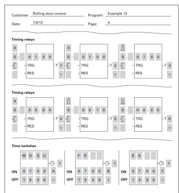
Figure 72. easyRelay Display Parameters
