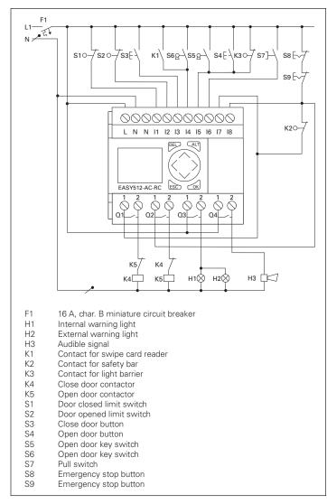
Figure 67. Control Wiring Diagram
