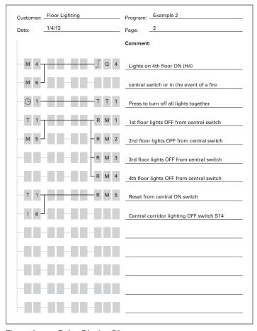
Figure 8. easyRelay Display Diagram
