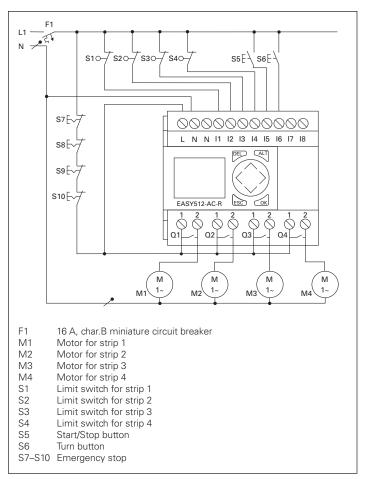
Figure 62. Control Wiring Diagram
