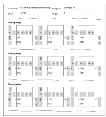
Figure 65. easyRelay Display Parameters
