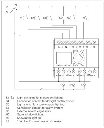
Figure 2. Control Wiring Diagram
