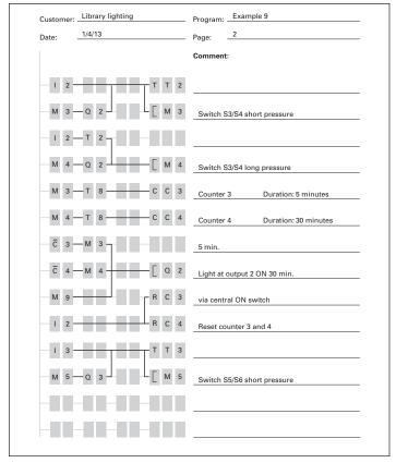
Figure 50. easyRelay Display Diagram
