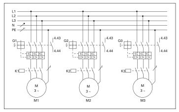
Figure 12. Load Circuit Diagram
