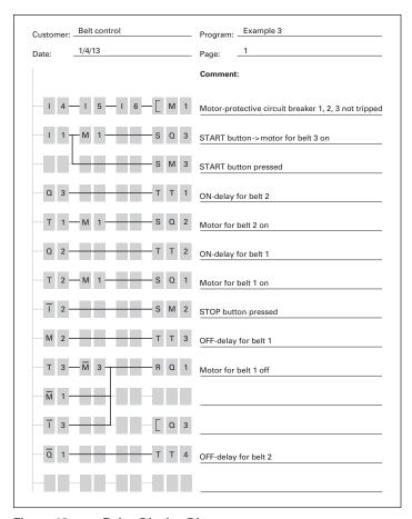
Figure 13. easyRelay Display Diagram
