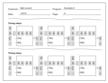
Figure 16. easyRelay Display Parameters
