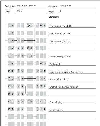
Figure 70. easyRelay Display Diagram
