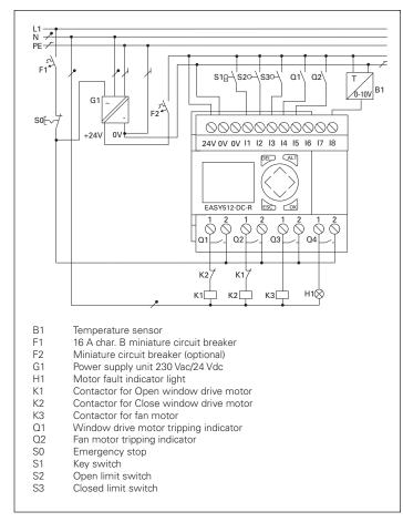
Figure 18. Control Wiring Diagram
