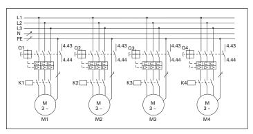
Figure 57. Load Circuit Diagram
