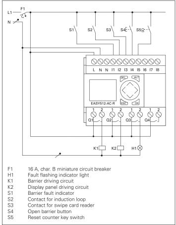
Figure 44. Control Wiring Diagram
