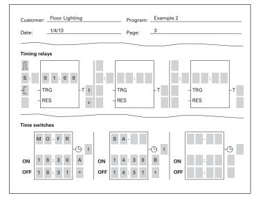
Figure 9. easyRelay Display Parameters
