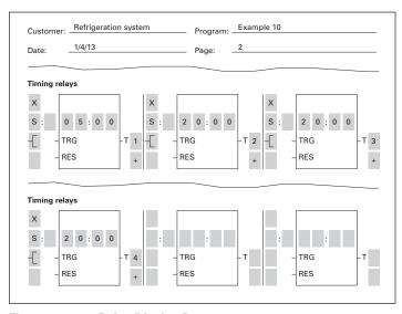
Figure 59. easyRelay Display Parameters
