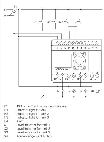
Figure 39. Control Wiring Diagram
