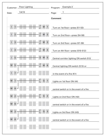
Figure 7. easyRelay Display Diagram
