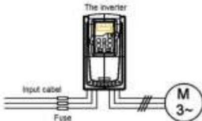
Figure 3-7 Fuse configuration
