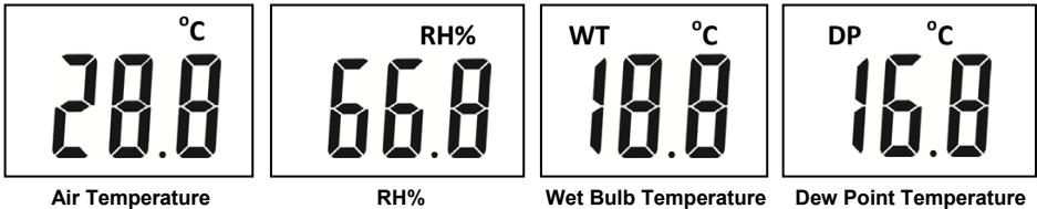
The meter runs the fan for 2 minutes upon power-up to generate readings; the meter only updates readings while the fan is running.
