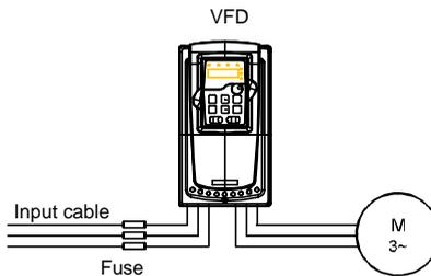
Figure 4-25 Fuse configuration
