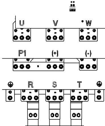
Figure 4-17 Main circuit terminals for the 355G/400P–500G models
