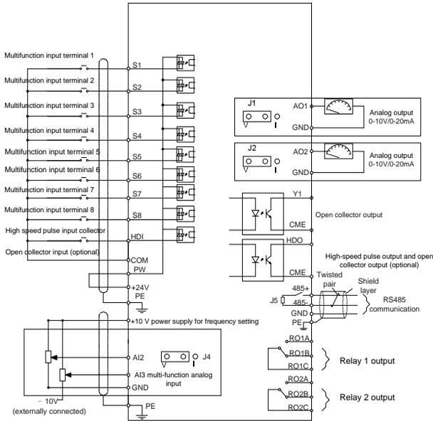
Figure 4-19 Wiring diagram of the control circuit
