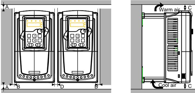
Figure 4-3 Parallel installation
