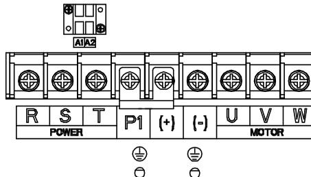
Figure 4-13 Main circuit terminals for the 037G/045P-055G/075P models
