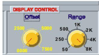
**Example 1:** Set the Offset by clicking and dragging the red indicator to "0000" (Diagram R-1). The screen shows 0001 as the starting point for the 8,000 record total.
