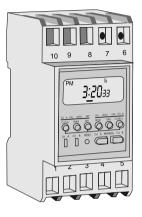
This electronic 7-day timer is accurate to the minutes, and has the capacity to accept up to 4 ON/OFF for CHANNEL 1 and 3 ON/OFF for CHANNEL 2, and can be set to repeat the daily programs 15 different ways as below. Each channel can be operated independently. You can choose to use one channel only or both channels together.
