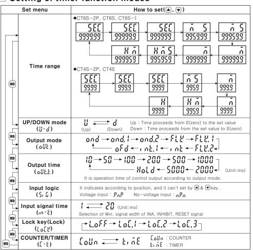
When setting the function mode, no external input signal will be accepted and the output will stay in the OFF state. \*\*In case of output mode is FKL, INT, INT1, OFD, there is no output time setting in the function setting mode. \*In the indicator type (CT6S-I), there are no the output mode and the output time setting mode(OUT1, OUT2) in the function setting mode.
