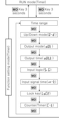
\*After selecting Timer in Counter/Timer of Counter function setting mode, if press MD for more than 3sec., it will move to Timer RUN
