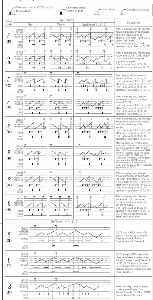
\*Output of single preset type is operating the same as OUT2 of double preset type
