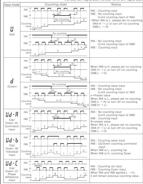
\*When use A,B phase of encoder with connecting to INA, INB, please set counter input mode as phase different input(Ud-C).
