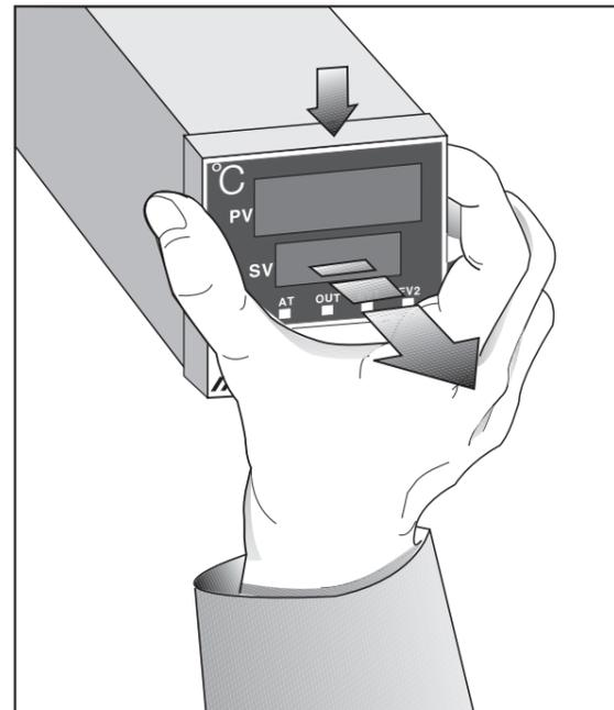
\*How to take out the inner body from the case : Pull the front panel guide to forward on pushing it to down direction.
